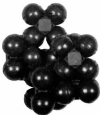
Fig.10. Cubic Im\bar{3} structure simulating the crystal structure of N_2O_4 (model 2d).
