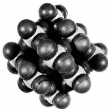
Fig.13. Cubic I\bar{4}3m structure simulating the crystal structure of SiF_4 (model 3b).
