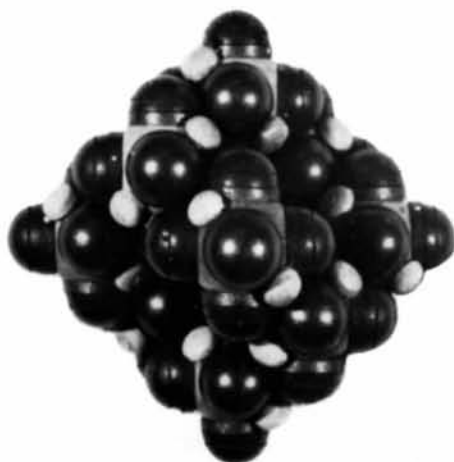
Fig.22. Cubic Fd\bar{3}m structure or diamond structure simulating the crystal structure of As_4O_6 and Sb_4O_6 (model 4d).
