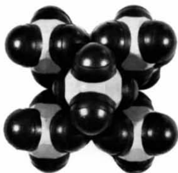
Fig. 15. Tetragonal P4_2/nmc structure simulating the crystal structure of B_4Cl_4 (model 3c).
