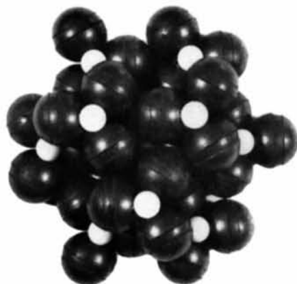
Fig.11. Hexagonal P6_3/m structure simulating the crystal structure of BCl_3 , BBr_3 and BI_3 (Model 2e).
