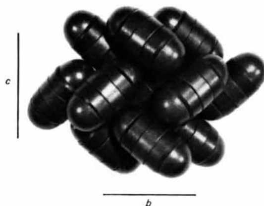
Fig. 5. Orthorhombic Pbca structure simulating the crystal structure of cyanogen (model 1c).
