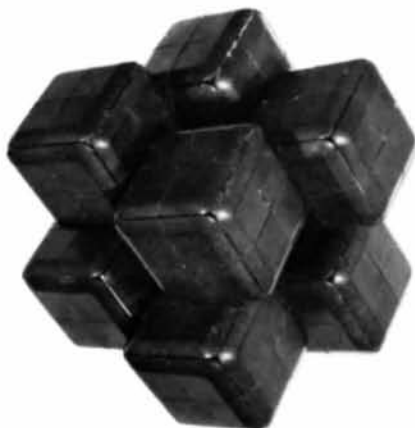
Fig. 19. Rhombohedral R\bar{3} structure simulating the crystal structure of (HSi)_8O_{12} and (CH_3Si)_8O_{12} (model 4a).
