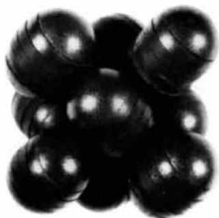
Fig. 2. Cubic Pa3 structure simulating the crystal structure of carbon dioxide (model 1b).
